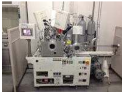
Fig. 3. Coaxial Arc Plasma Deposition System
