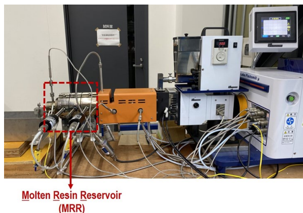
Fig. 1. Novel extrusion process with MRR unit.
