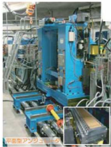
Number of periods: 24 Period: 85 mm Total length: 2016 mm Magnat size: 20x20x126W Remnant Field: 1.2T Deflection parameter K: 3.6 - 0.54 (gap 31 - 80 mm, hv 14 29 - 207eV)
